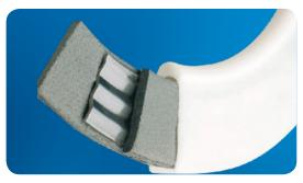
Glass Lined Vessel Gaskets compose of a PTFE envelope, PF2000LR CNAF aramid fibre insert & corrugated stainless steel ring all of which are manufactured under one roof.
