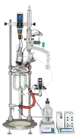
Since we at NORMAG always rely on widespread standard flanges and cuts, we can also use existing accessories. Just as future-oriented and customizable is the associated control and data storage CU Pro2, which can be coupled with many laboratory devices (pumps, scales, ...), sensors and actuators.
