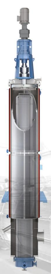
Our mobile pilot Wiped Film Evaporator (WFE) unit was sent to the customer's site to perform the trials to prove the concept and collect data for scale-up.
